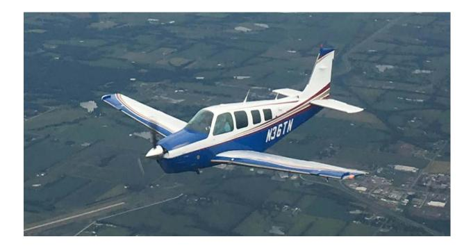
The new Gross Weight Increase (GWI) approval is available on certain Beechcraft Bonanzas configured with an IO-550B engine and two of GAMI's STC'd modifications including *GAMIjector*® fuel injectors and components of their *Liquidair*<sup>TM</sup> Baffle Kit. The GWI ranges from 180-300 lbs. based upon aircraft model.
