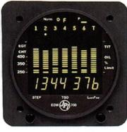
FIGURE 2: E.I.'s US-8 Ultimate Scanner displays absolute digital EGT information, as does JPI's EDM-700, and subsequent generations of digital engine monitors have all done the same.
