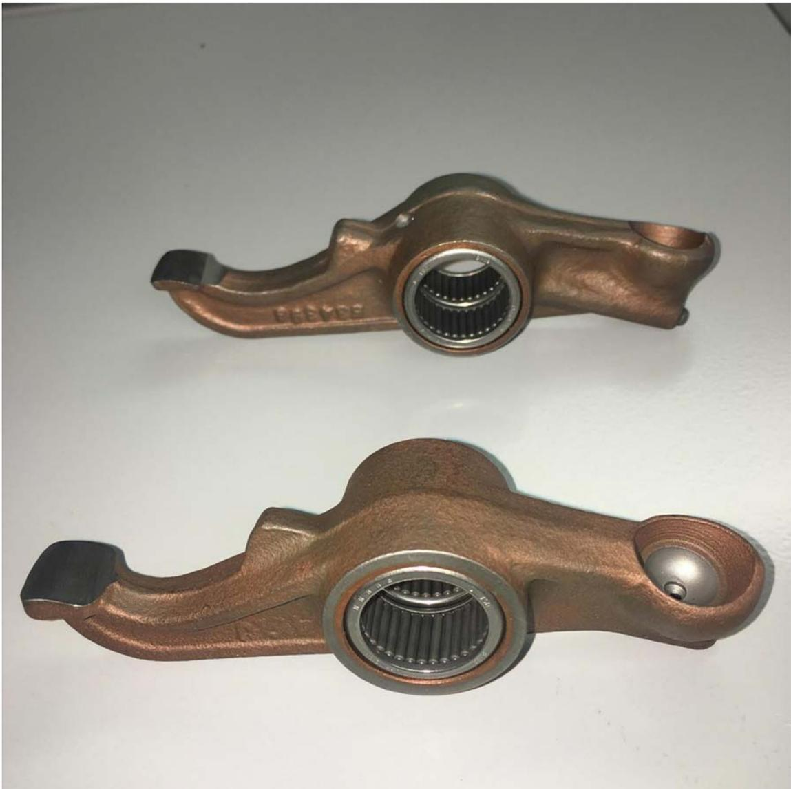
**The *Needle Bearing Rocker Arms* are approved for use on specific models of IO-470, IO-520 and IO-550 engines, both naturally aspirated and turbonormalized. Availability is targeted for the summer of 2019.**
