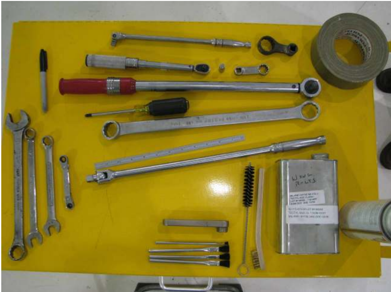
Fig. 2 Tools & supplies required for ALEC cable installation.
