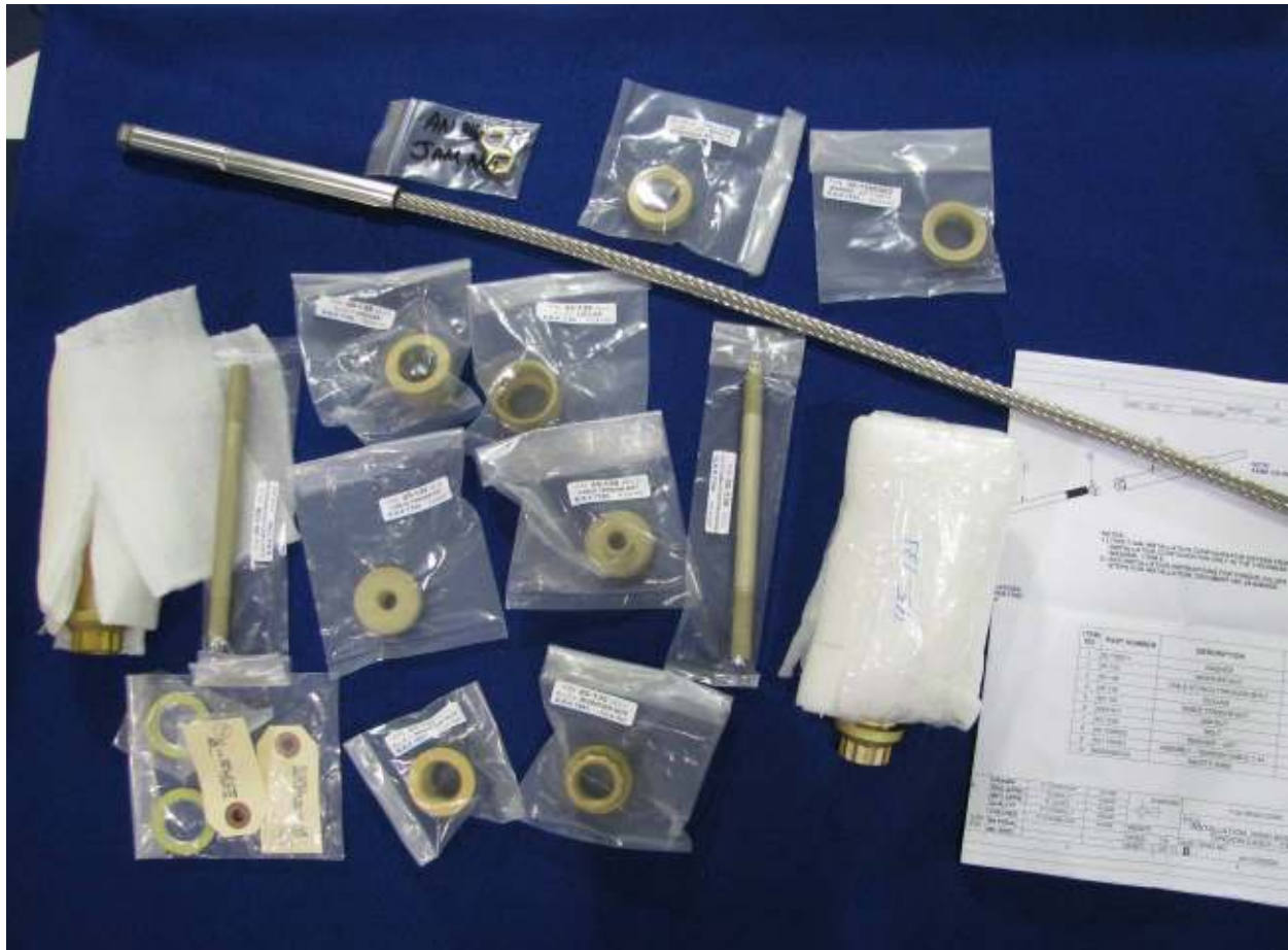
Fig. 3 ALEC parts to be installed on T-34 and T-34A aircraft. T-34 B is identical except the washers under the head of the wing bolts are 0.25” thick, rather than 0.43” thick for the A model.
