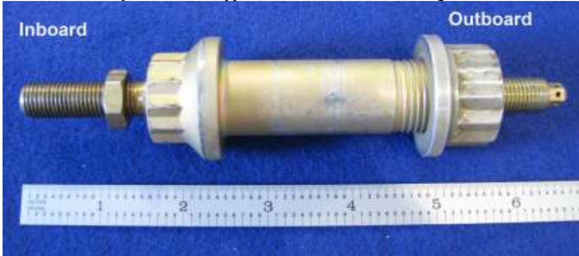
Fig. 6 Install one 45-136 Through Bolt and AN316-7 jam nut in position oriented as shown. This is done by inserting the Through Bolt into the lower access with the inboard side first and then manipulating the outboard end of the Through Bolt through the head of the newly installed Wing Bolt and then moving the Through Bolt outboard so that the end protrudes into the bathtub fitting area. After this is in place, and from the same side, insert cable/Through-Bolt assembly (see Fig 6a to 6f) from the same side with the Through-Bolt first. Through-Bolt is then routed through the entire center section. Then remove thread protection and manipulate the tip of the Through Bolt to pass it out through the open hole in the Wing Bolt on the opposite side.
