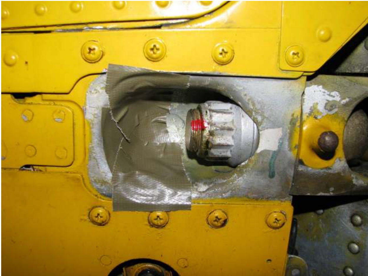
Fig. 4 Protective tape in place to protect bathtub fitting.
