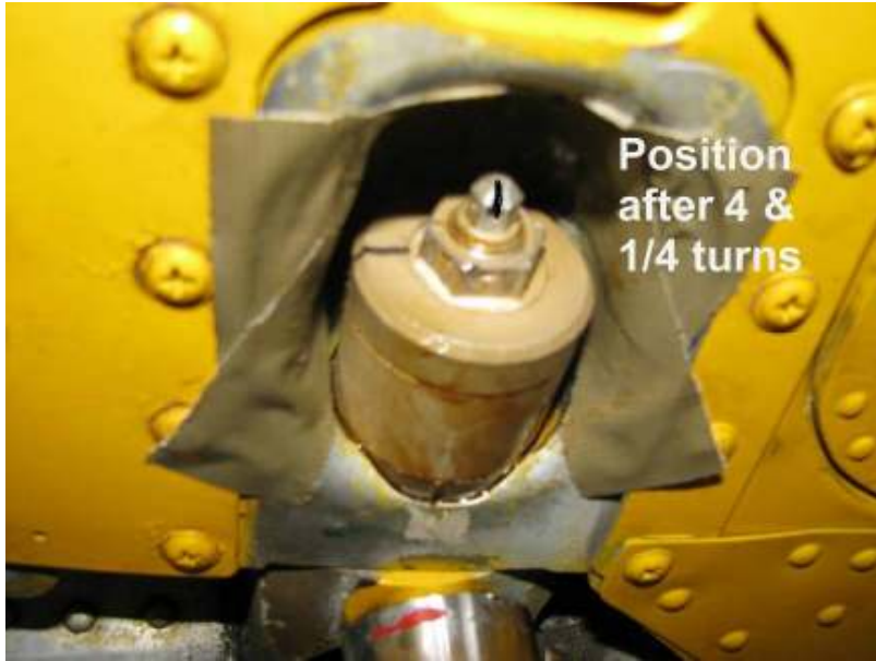
Fig. 10 Tension Nut after 4 \frac{1}{4} turns (continue rotating tension nut an additional \frac{1}{4} turn).
